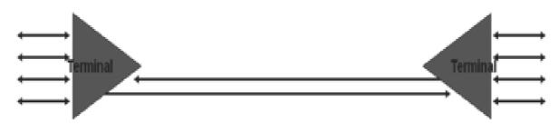
A lone system is system to the PDH network topology. Traffic is added and dropped only at the end points of the network. Terminal nodes are used at the end of the network for adding and dropping the traffic.
